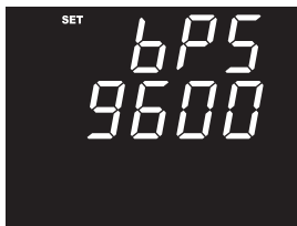
Figure 3-32 Communication baud rate setting
