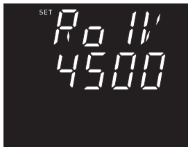
Figure 3-54 RO1/DO1 alarming setpoint setting
