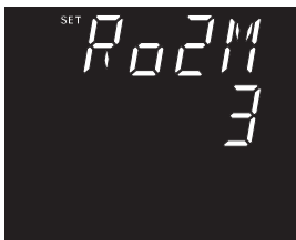
Figure 3-57 RO2/DO2 working mode setting
