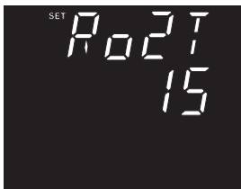
Figure 3-60 RO2/DO2 alarming delay time setting
