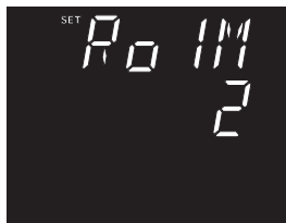
Figure 3-52 RO1/DO1 working mode setting
