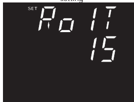
Figure 3-55 RO1/DO1 alarming delay time setting
